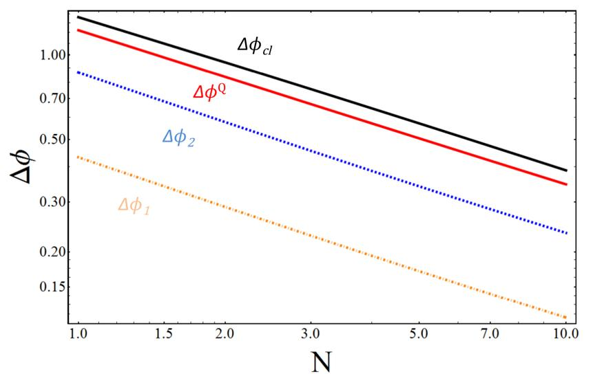
Best precision for optimal  $\tau$  and with losses as a function of total photon number. In such case  $\Delta\phi_Q \neq \Delta\phi_{cl}$ . For  $\Delta\phi_1, \Delta\phi_2, \tau=0$ , for  $\Delta\phi_Q, \Delta\phi_{cl}, \tau=0.5$ .
