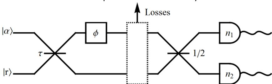
$$F_{cl} = \sum_{n_1, n_2} \frac{1}{p(n_1, n_2 | \phi)} \left( \frac{dp(n_1, n_2 | \phi)}{d\phi} \right)^2, \quad \Delta\phi_{cl} \geq \frac{1}{\sqrt{F_{cl}}}$$
