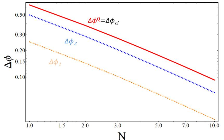
Best precision for optimal  $\tau$  and without losses as a function of total photon number. In such case  $\Delta\phi_Q = \Delta\phi_{cl}$ . For  $\Delta\phi_1, \Delta\phi_2, \tau=0$ , for  $\Delta\phi_Q, \tau=0.5$ .
